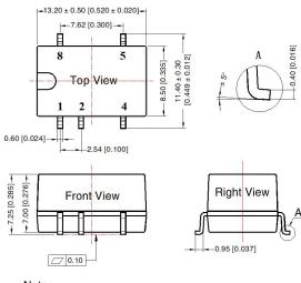
Note: Unit: mm[inch] Pin section tolerances:  $\pm 0.10[\pm 0.004]$ General tolerances:  $\pm 0.25[\pm 0.010]$
